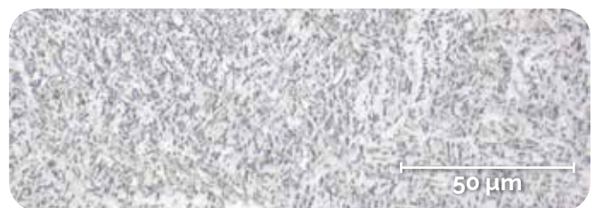
Figure 6: A higher resolution image of a sample manufactured through TiMIM + TiRx.
