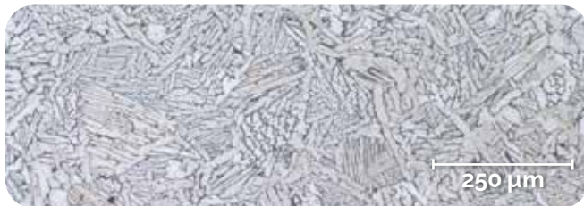
Figure 3: TiMIM sample. Virtually no grain boundary alpha is present, and the grains are finer and more equiaxed than those created during investment casting.
