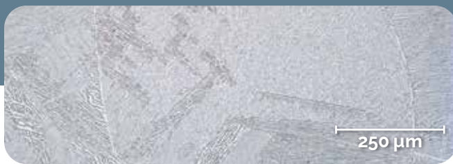
Figure 1: Typical cast titanium microstructure. The white at the grain boundaries is aggregated alpha phase, which is more brittle.
