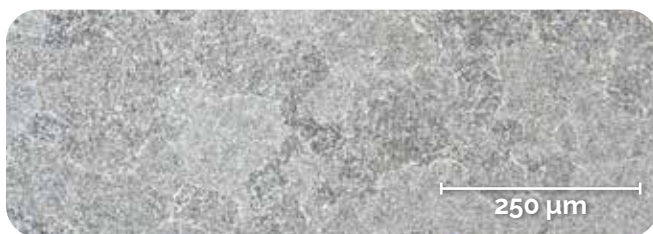
Figure 5: TiMIM + TiRx. Very little grain boundary alpha, and finer, more equiaxed grains.
