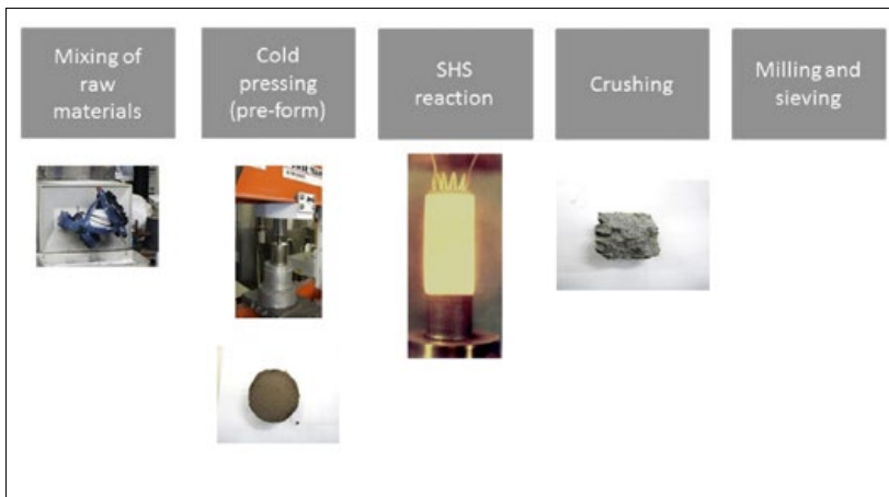
Fig. 9 Production scheme of reinforcement particles [10]
