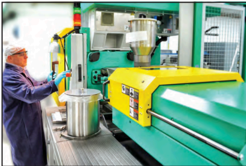
Figure 1. All-electric injection molding machine in an ISO 13485 environment
