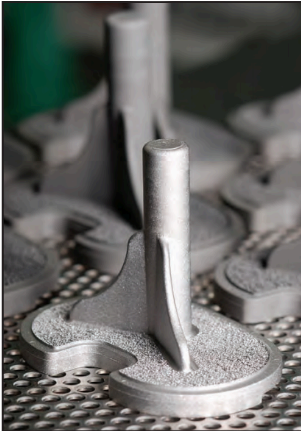
Figure 2. Ti-6Al-4V MIM orthopaedic implant with porous ingrowth features
