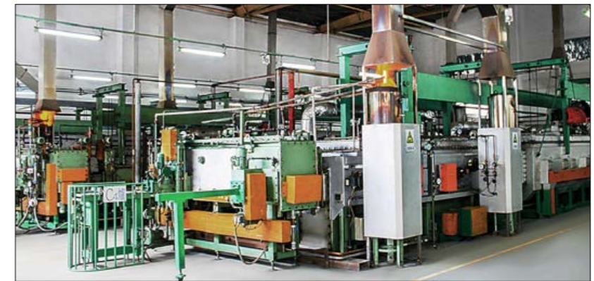
Fig. 3 Continuous MIM debind and sintering furnaces in operation
