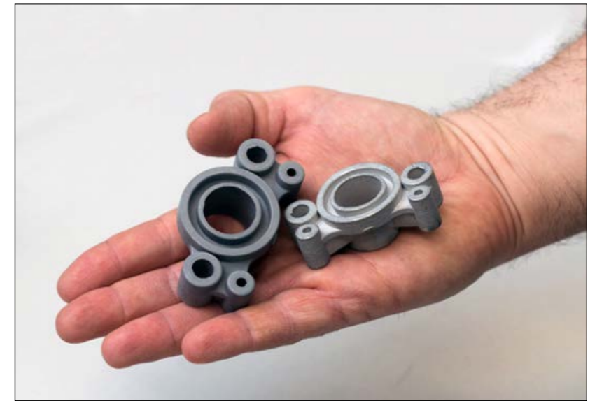
A green aluminium MIM part, left, and the sintered part on the right
