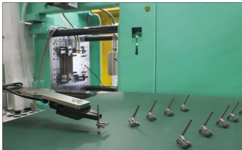
Fig. 2 Automatic part removal at Vibrom using Arburg's Multilift H system linked to an Allrounder 370S injection moulding machine
