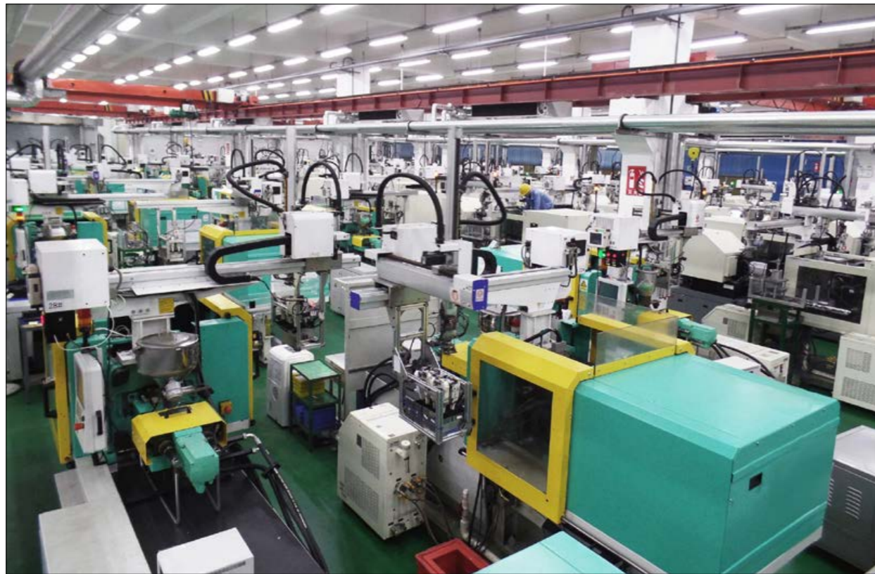
Fig. 2 Zoltrix operates more than 250 injection moulding machines for MIM production, many with automation to facilitate high volume production
