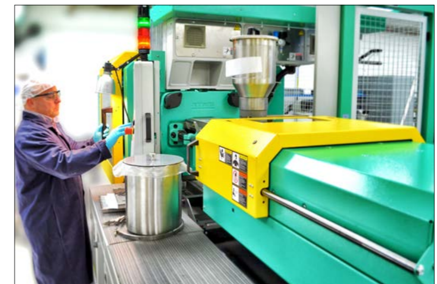
Fig. 1 Injection moulding of TiMIM parts at Praxis Technology
