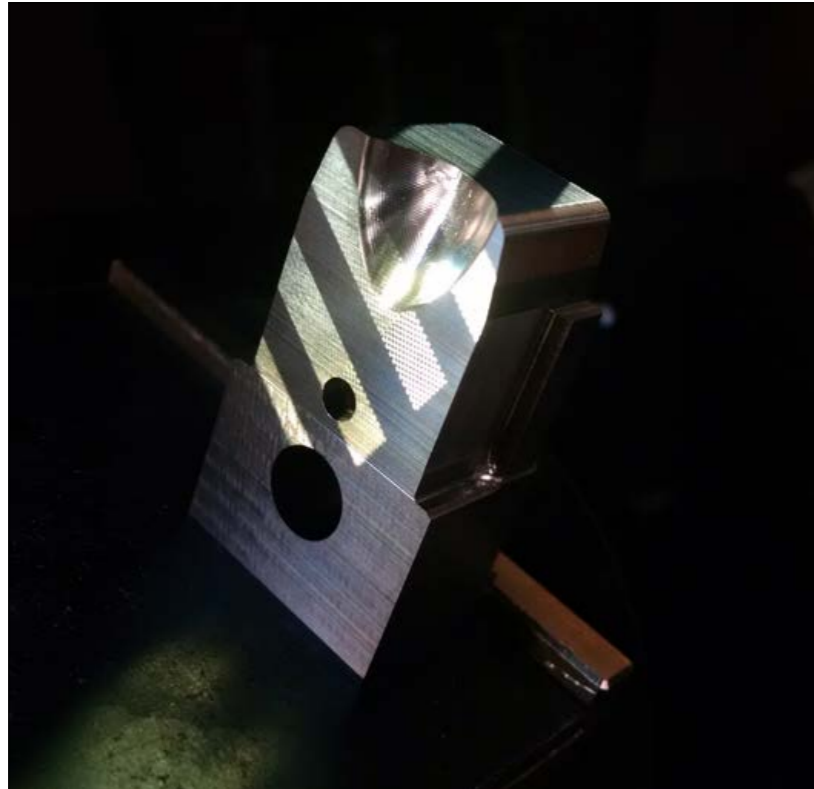
Fig. 4 A 3D inspection system that utilises structured light is used at Dynamic Group
