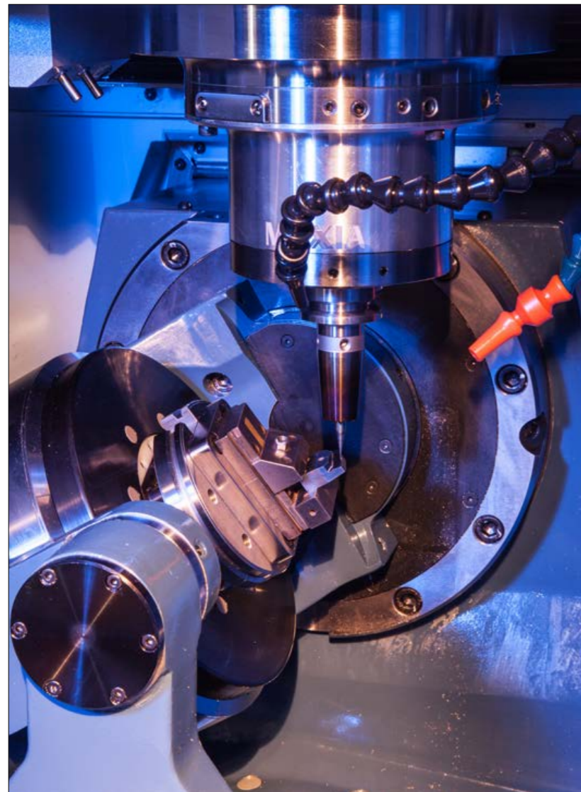
Fig. 7 Detail view of one of the two Matsuura 5-axis high speed high precision milling machines at Dynamic Group (as seen in the background of Fig. 2)
