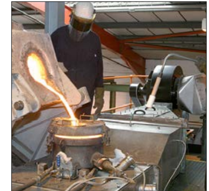
Powder production underway at Atomising Systems Limited
