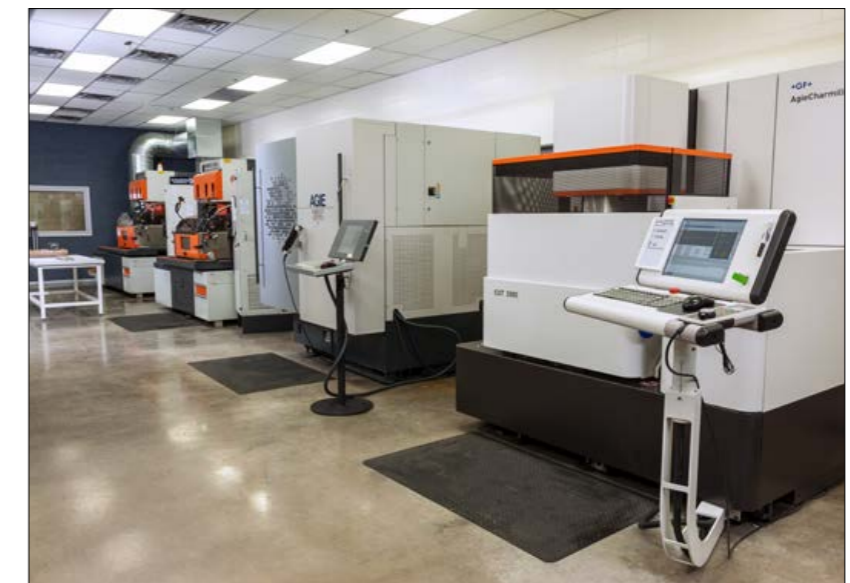
Fig. 1 Part of Dynamic Group's injection mould manufacturing facility in Minneapolis showing various wire EDM machines
