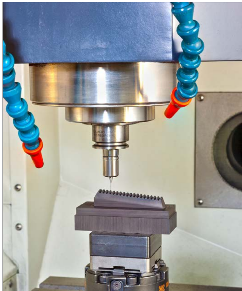
Fig. 10 All electrodes are produced on System 3R pallets and manufactured in one of two dedicated and identical Makino machining centers at Dynamic Group
