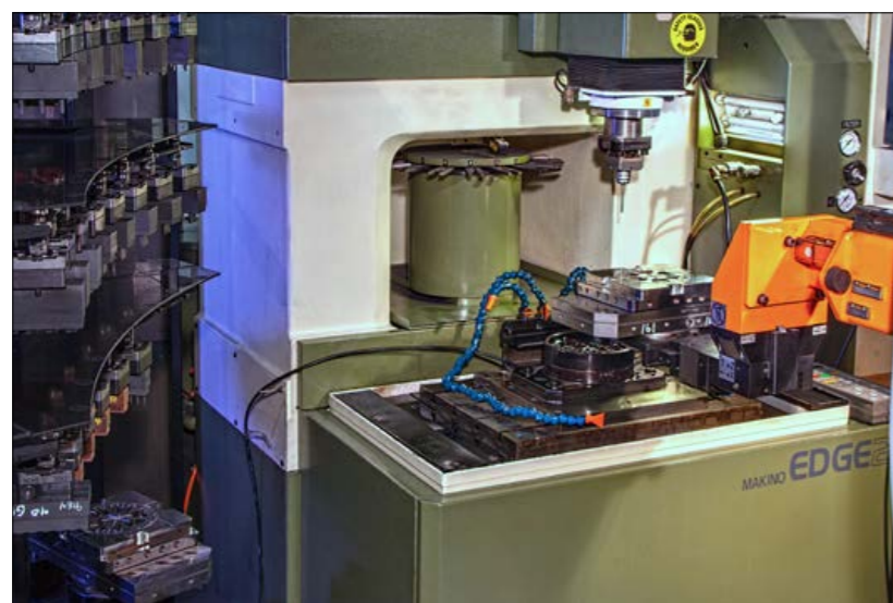
Fig. 8 Detail of a Makino Edge 2 precision sinker EDM machine with horizontal robot
